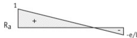
Figure 3 - Influence line for the support reaction at A
