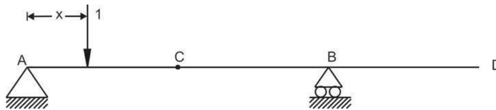
A unit load before section C
